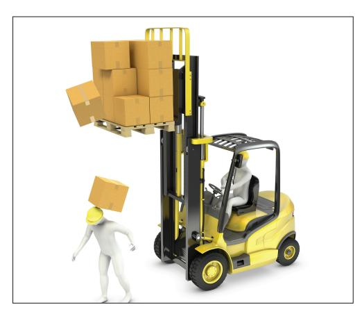
Load handling presents an additional set of hazards to operators. Off-center loads, overloading, and damaged or loose loads can all cause tip over or falling loads and collisions if the
