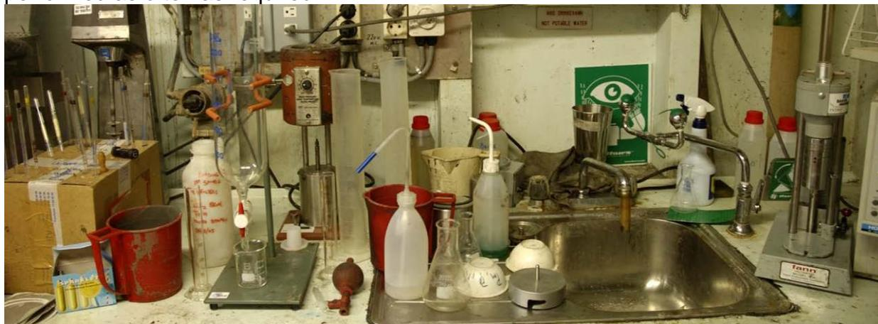
**Can you find the eyewash? In the real world, eyewash stations are often badly marked, difficult to find, and difficult to operate fast in a panicked state, falling short of the real safety goal of treating eye burns quickly.**
