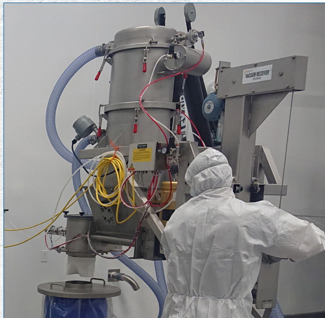
VAC-U-MAX Sanitary Vacuum Conveyor mounted on rolling frame allows mobility and equipment access.
