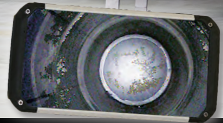
Video image of confined space area displayed on a 5" tablet
