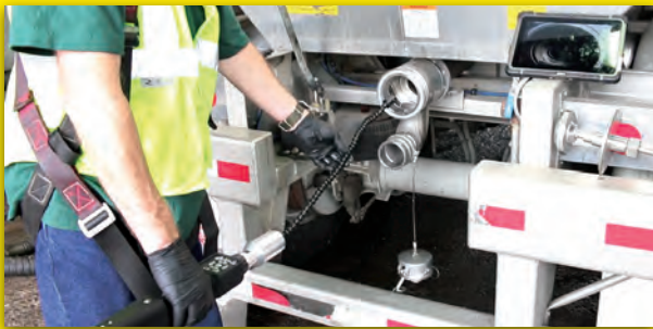
Valve Inspection Camera in use with 10" rugged display
