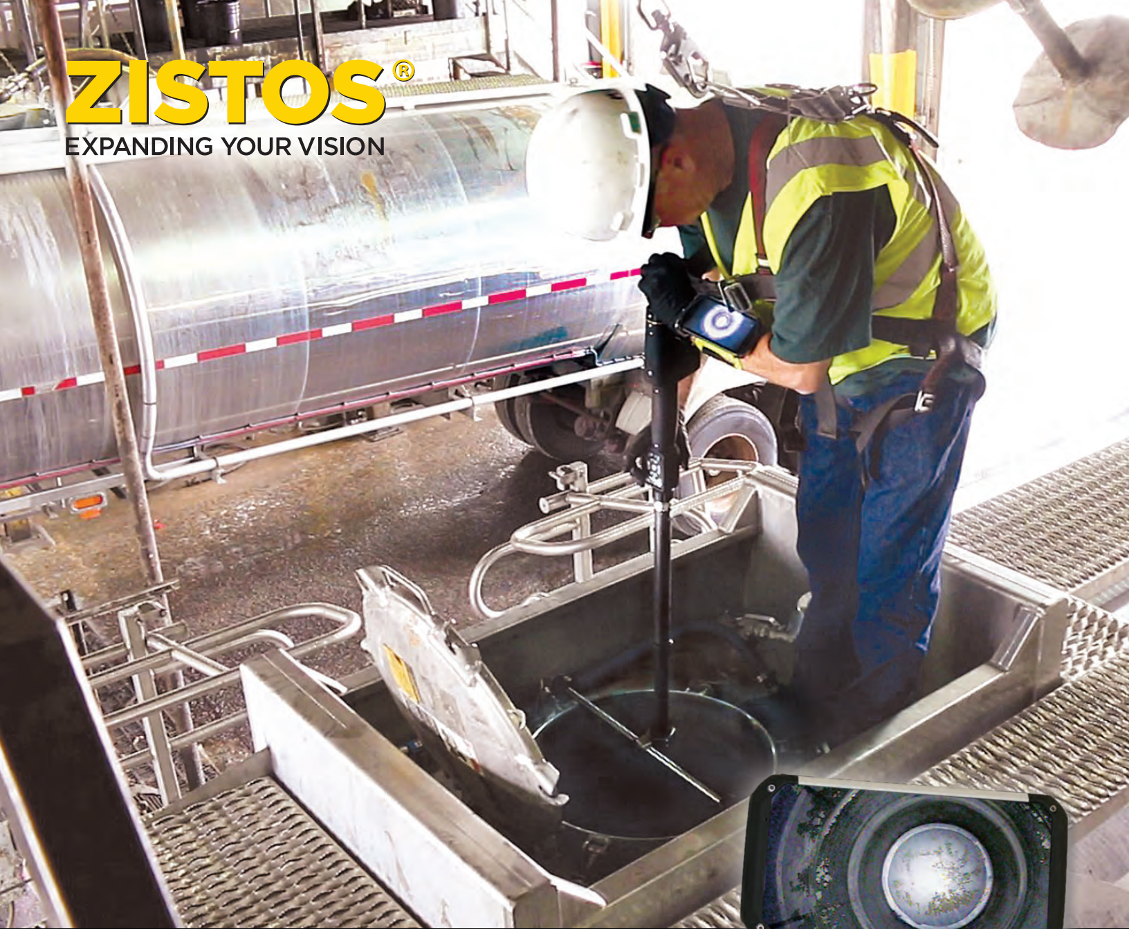
Video image of confined space area displayed on a 5" display
