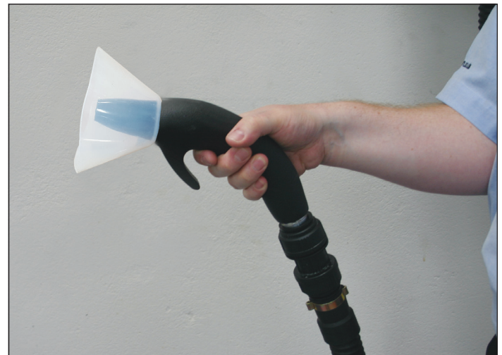
Chip guard attachment enhances operator safety
